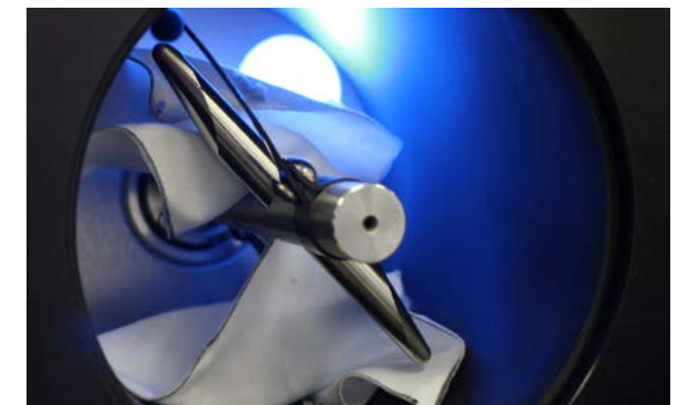
The air circulation is specifically engineered to keep the specimens tumbling for the duration of the test.
