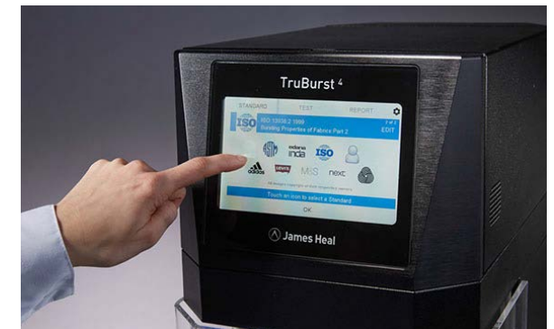
The on-board software enables TruBurst to be operated independently of a PC for bursting strength testing.
