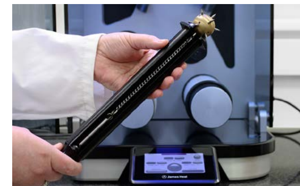
The Mace Ball Holder holds the mace ball safely and securely for inspection of the points for wear or damage as specified in VDA 230-220.
