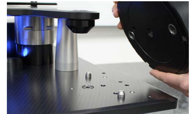
The removable table enables specimen material to be positioned and secured away from the instrument.
