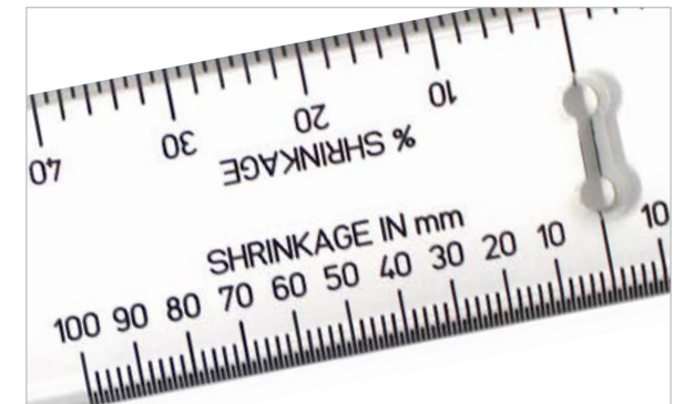
The James Heal stretch and recovery ruler measures percentage stretch and recovery without calculation.
