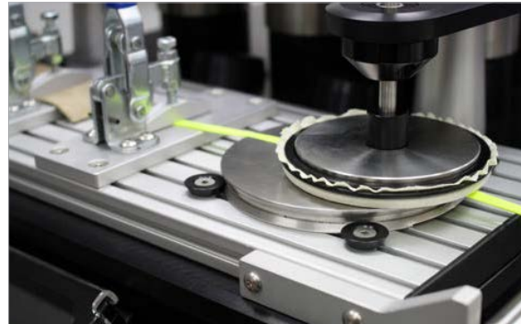
A table assembly is attached across the base plate to test abrasive properties of multiple types of straps, ropes and shoelaces .
