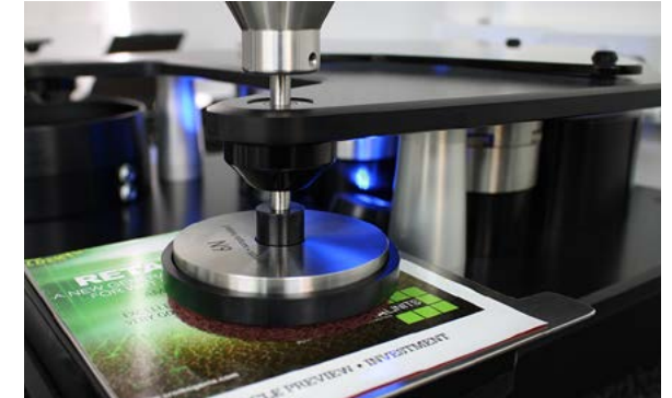
After testing the specimen mounting plate can be taken to an assessment cabinet without the need for further handling.
