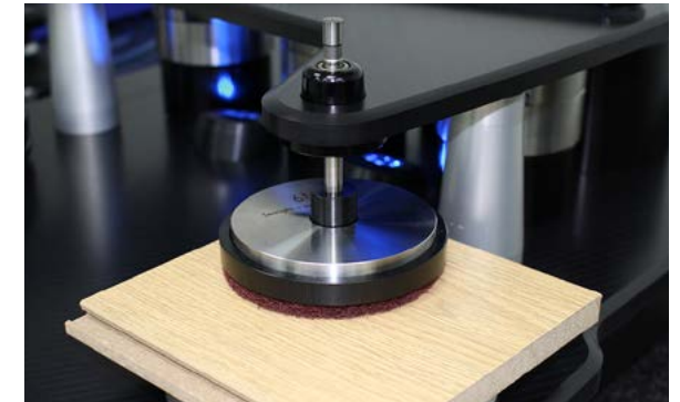
Fully compliant with EN16094, once tested the results are simple to grade.
