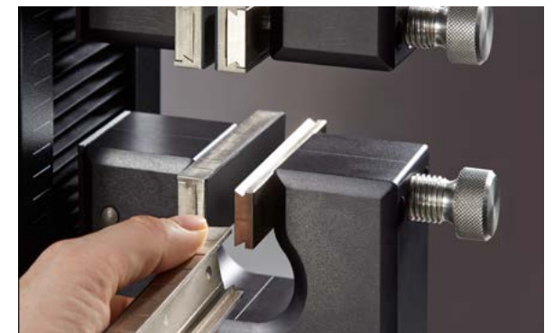
The simple and tool-free process for changing the jaw faces is one of many features of our Titan instruments to enhance ease of use.
