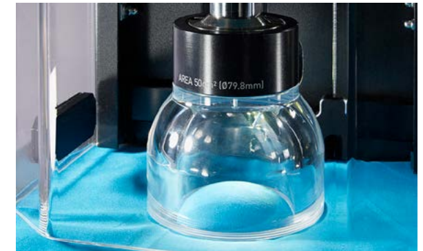
Accurate contactless laser distension measurement ensures pin point accuracy and extended diaphragm life.
