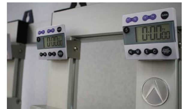
Each station has an independent timer which can be used in position or remotely, which minimises user downtime.
