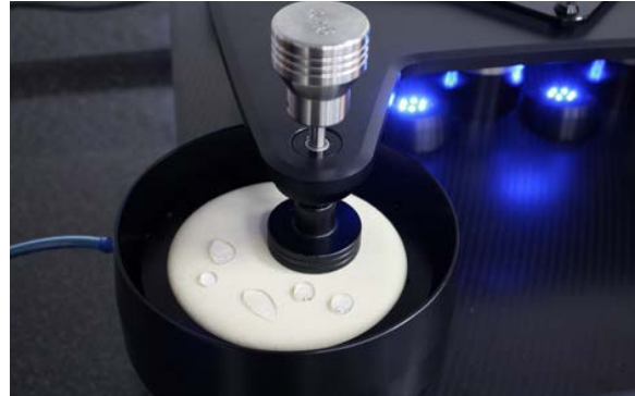
The water bath option is used to test products while damp or fully submerged in water.
