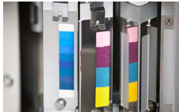
Our tri-sided sample holders are really easy to load and unload, and offer up to 1640cm 2 of usable exposure space.
