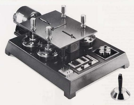
Circular specimens of fabric are rubbed against a standard abradant, under a known pressure, and the resistance to abrasion is determined by the number of rubs to breakdown or by the loss in mass of the specimens.
