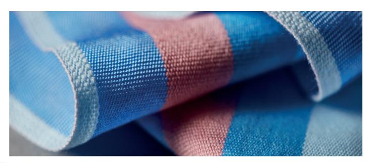
We weave our Multifibre DW internally, carrying out a consistent testing process to ensure you receive a consistently high-quality test fabric. The materials composition is compliant with the requirements specified in ISO 105 F10 and is approved by many leading UK and European specifiers.
