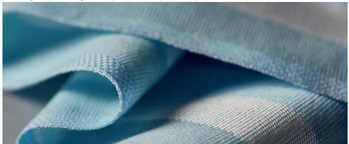
Our internally woven Multifibre LW is approved by a number of UK retailers including Marks & Spencer. It has a similar composition to the Multifibre DW variation but with the acetate strip replaced by the regenerated cellulose strip. This helps make the product more reflective of the fabrics found in current apparel.
