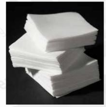
The crocking test is based on assessing the amount of dye transferred from the specimen under test to a standardised crocking cloth.
