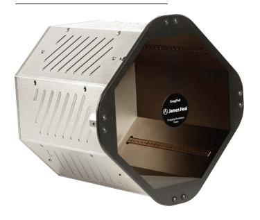
James Heal led the development of the SnagPod to solve the problem of testing for undesirable loops on the surface of garments, for which a suitable method did not exist.
